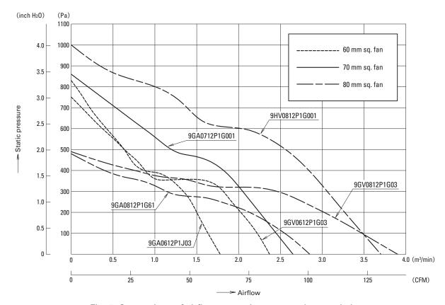
Fig. 5: Comparison of airflow vs. static pressure characteristics
