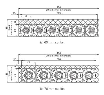
Fig. 6: Installation on a 2U unit
