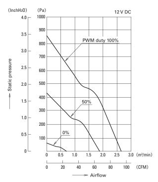
Fig. 4: Airflow vs. static pressure characteristics against PWM duty cycle (9GA0712P1G001)
