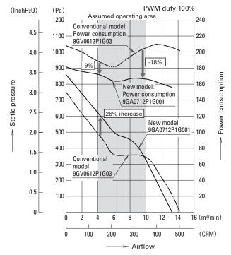
Fig 7: Airflow vs. static pressure characteristics of the conventional and new models (Six 9GV0612P1G03 units or five 9GA0712P1G001 units in parallel)
